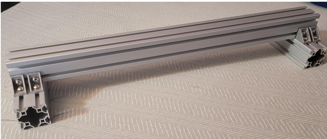
*Figure 3: Aluminum 80/20 Extrusions*
